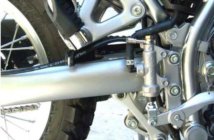
**a. Rear master cylinder, Galfer line routed through OEM routing clip**
