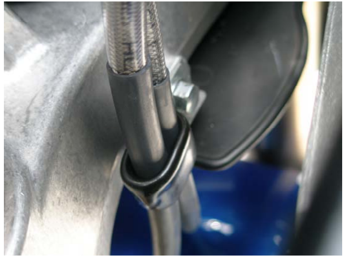
b. Galfer c-clip at lower triple tree
