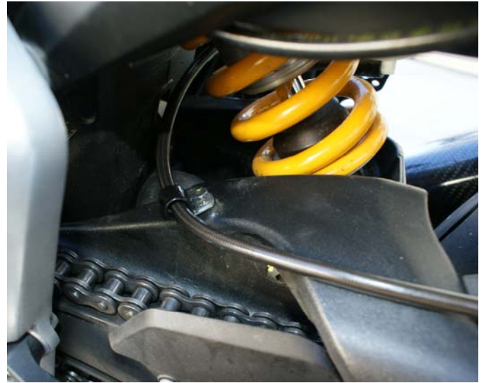
B. Galfer line running behind shock and through c-clip at swing arm
