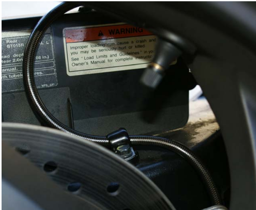
E. Close up of Galfer line and c-clip at inner swing arm
