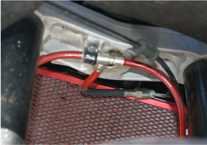
**E. Galfer Line at OEM Hard Tubing and Galfer C-Clip at Lower Triple Tree**
