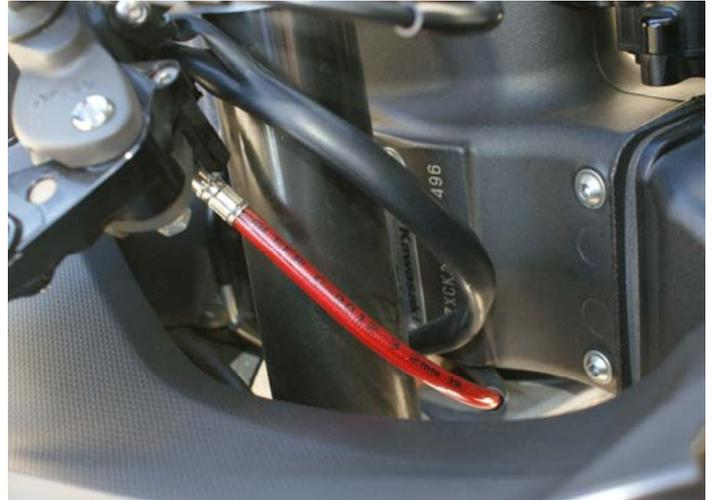
**B. Master Cylinder Line Routing**
