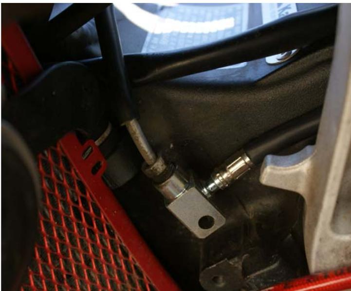
**C. Master Cylinder Line at Right OEM Hard Tubing.**
