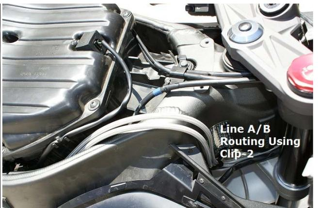
Picture 4 – Lines A & B Routing with Clip-2
