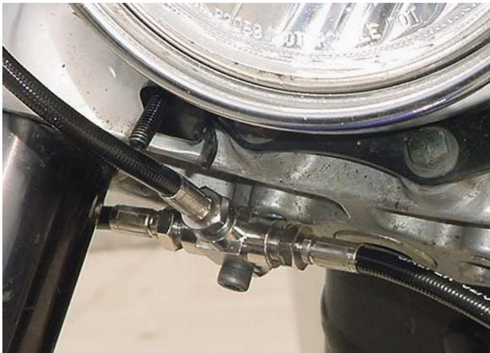
**c. Galfer t-block at lower triple tree**
