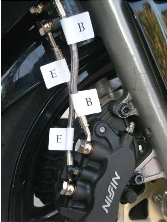
**e. Lines B & E from delay valve to right caliper**
