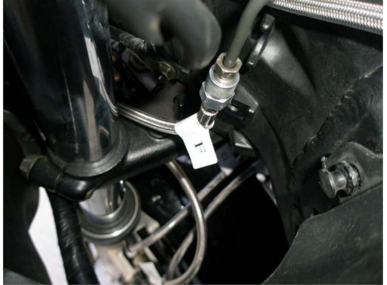
**r. Line F routed in front of the lower triple tree**
