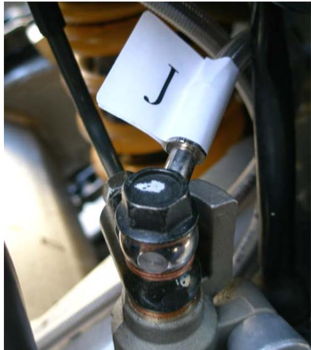
**v. Line J at rear master cylinder with OEM tubing and bolt**
