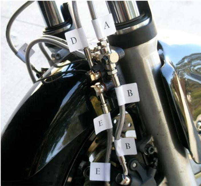
**c. Lines A, B, D & E at right caliper delay valve**
