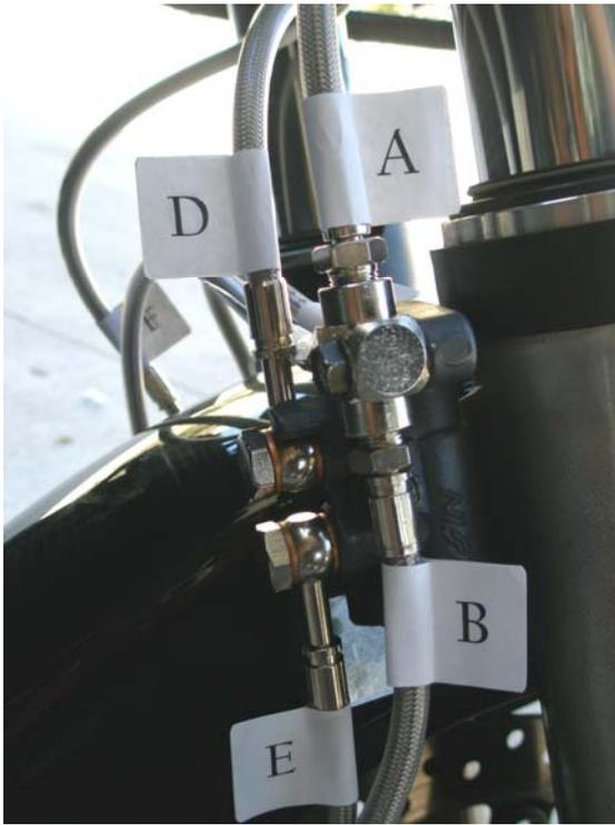
**i. Lines A, B, D & E at right caliper delay valve**
