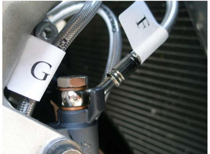
**l. Line F installed at left caliper secondary master cylinder
