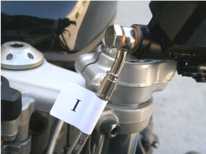
**s. Line I at clutch master cylinder**
