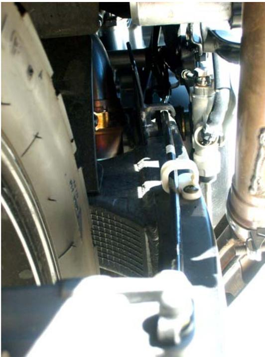
**c. Rear routing, using OEM routing clip**
