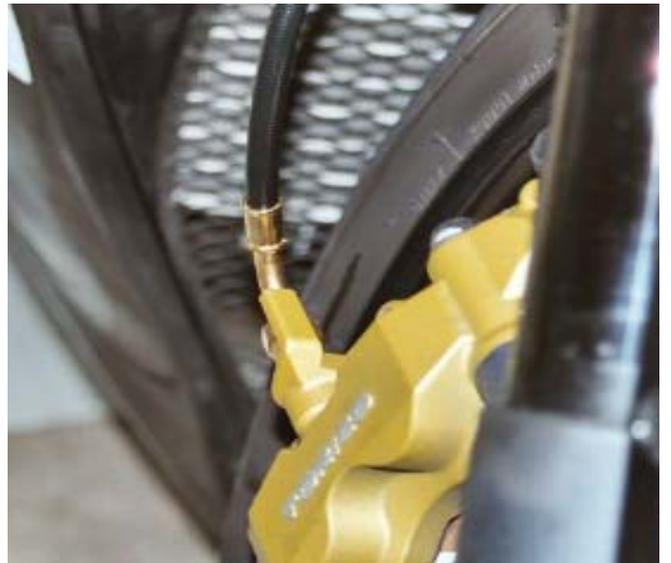
**D. Note: the position of the brake line is slightly away from the bike**
