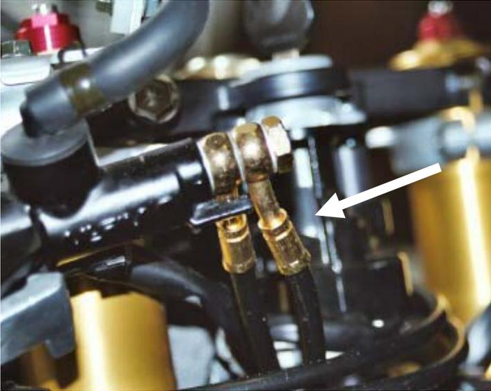
**A. Master Cylinder (Note: the left line is positioned slightly in front of the right line)**
