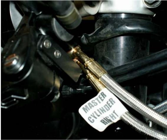
**a. Front master cylinder, notice positioning of left line**
