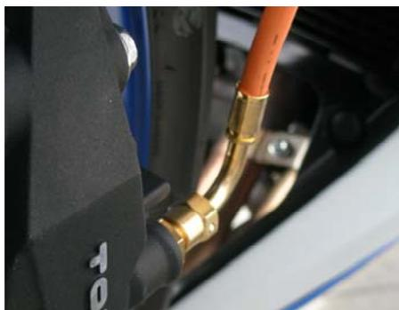
**e. Left caliper, notice fitting is pointing away from the bike**
