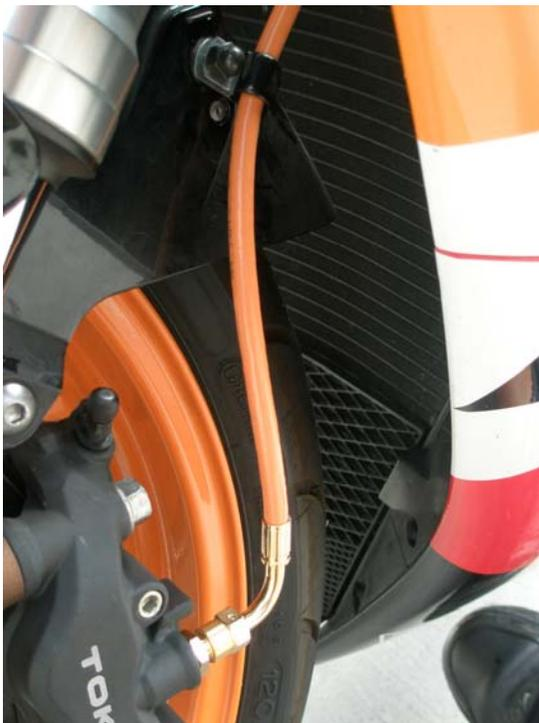
**g. Right caliper, notice Galfer provided c-clip at fender**
