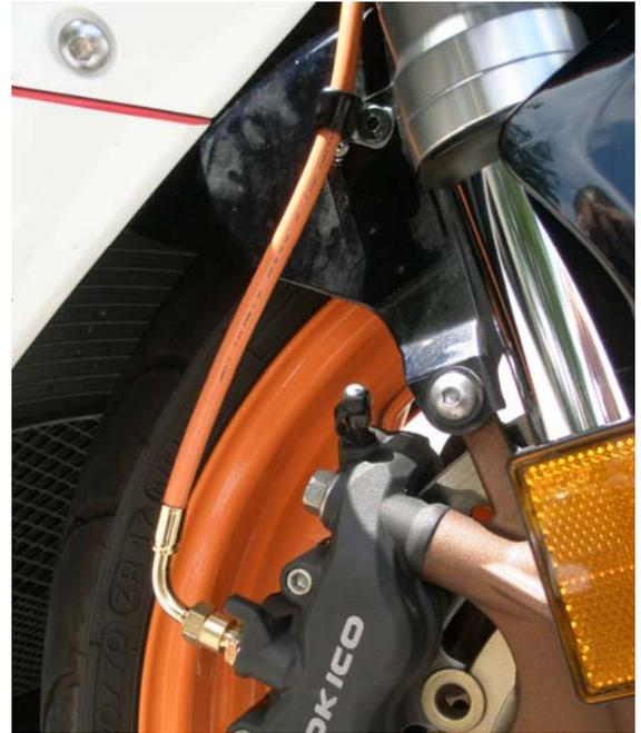
**f. Right caliper, notice Galfer provided c-clip at fender**
