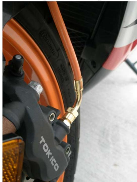
**h. Left caliper, notice position of fitting**
