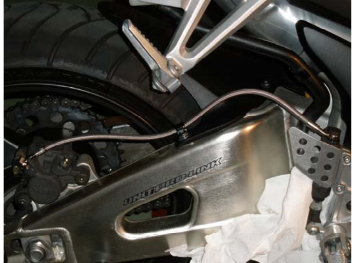
D. Overall Line Routing
