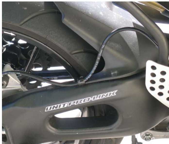
C. Galfer C-Clip at Swing Arm, Overall Line Routing
