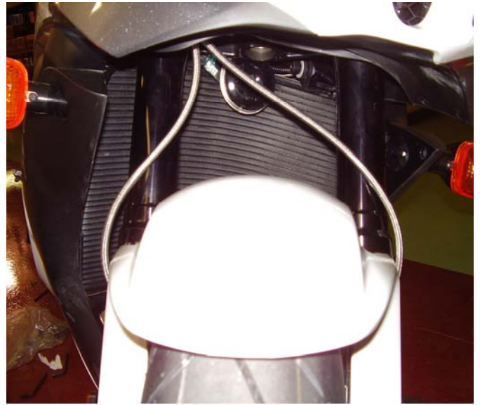
B. Overall Line Routing
