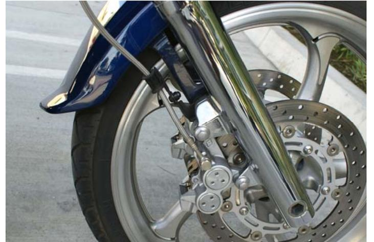
**d. Right line at right caliper and OEM line holder**
