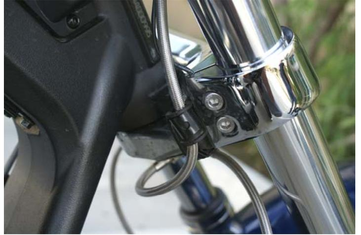
**b. OEM line holder at the lower triple tree**
