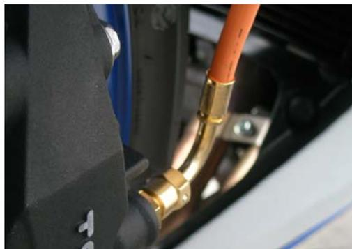
**e. Left caliper, notice position of fitting**
