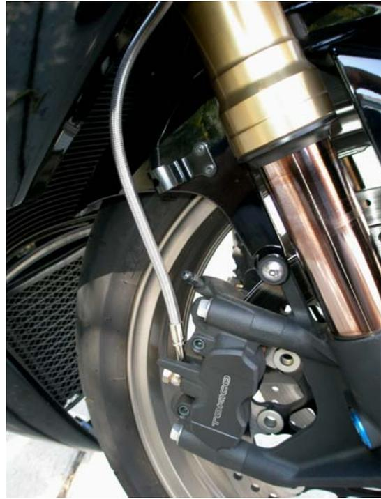
**f. Right caliper routing**
