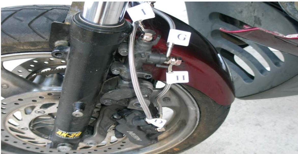
LEFT CALIPER / DELAY VALVE
