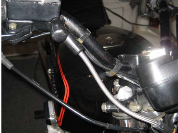
a. Front master cylinder, re-using OEM fitting cover
