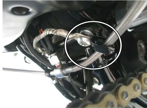
**b. Brake light switch from master cylinder, Galfer larger c-clip in circle**
