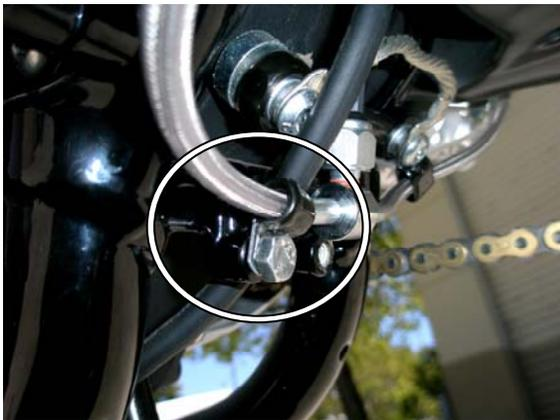
**c. Brake light switch to swing arm and caliper, Galfer altered c-clip in circle**
