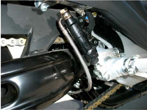
**a. Rear master cylinder and routing underneath bike**
