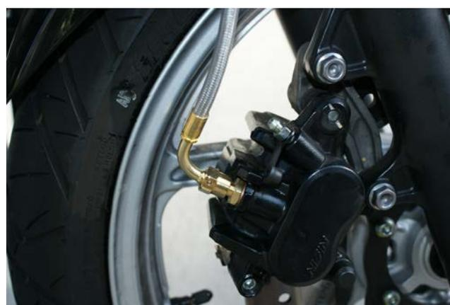
**f. Hex fitting and adapter at caliper**
