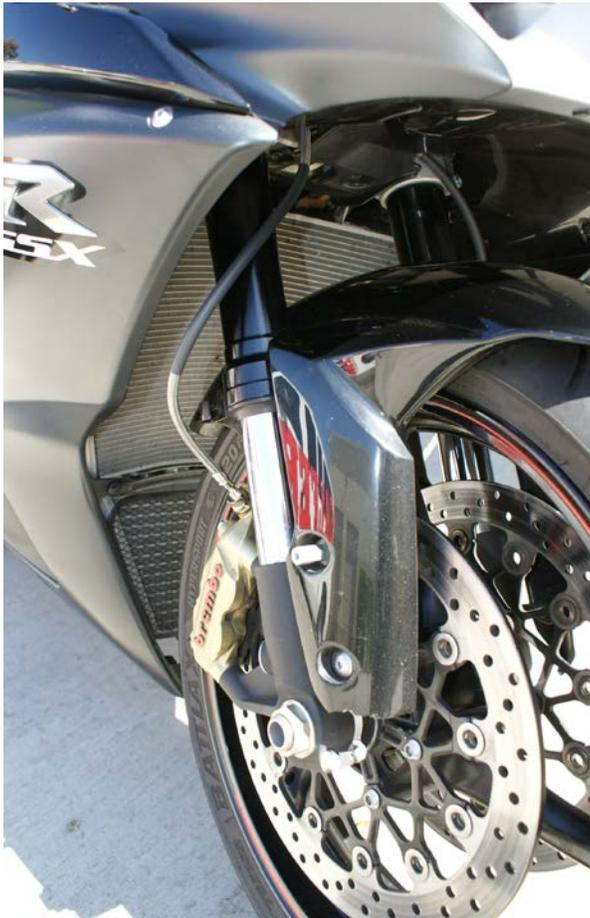
**C. Galfer Right line routing in front of forks**
