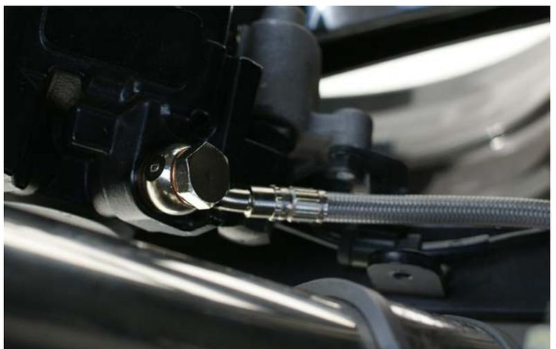
**n. Line E installed at rear caliper**
