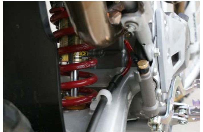
B. Routing through stock line holder on swing arm
