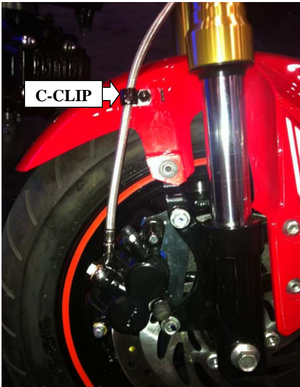
C. C-Clip at Fender & Line at Caliper
