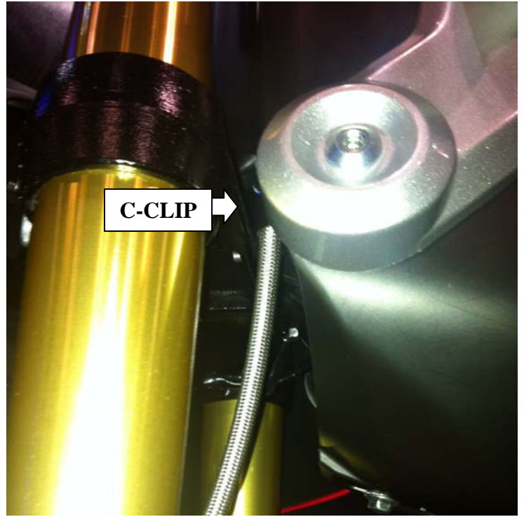
B. C-Clip & Brake Line at Triple Tree
