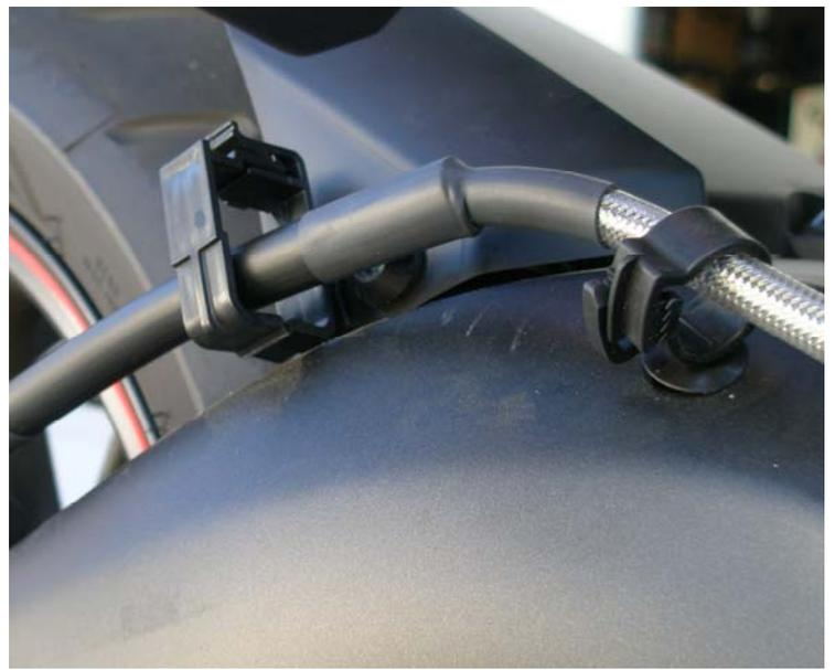
**B. Rear line through stock guide brackets**
