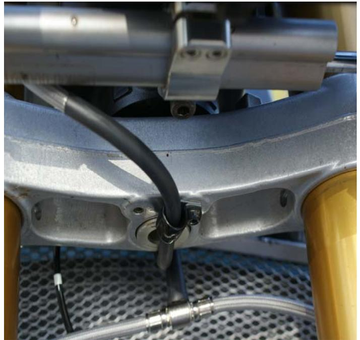
Line-A routing lower triple using
