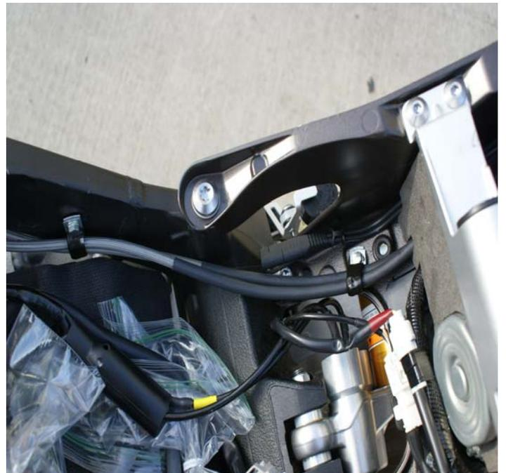
Line-A-D right frame routing to ABS Unit
