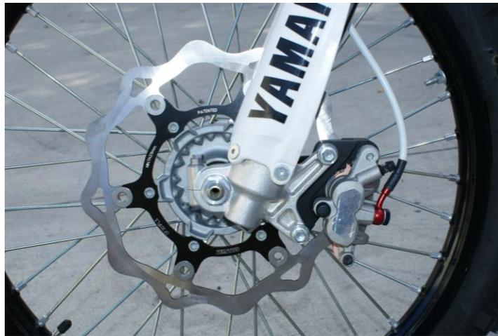
Be sure to pump the brake lever a few times, making sure the system is working properly. Please be aware that the overall braking feel has been changed dramatically. We suggest taking it easy while you get used to the new brake lever pressure and feel. If you have questions, do not hesitate to call our tech department – **1(800) 685-6633**.
