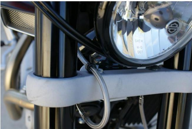
**b. Line A routed in front of lower triple tree, using c-clip**
