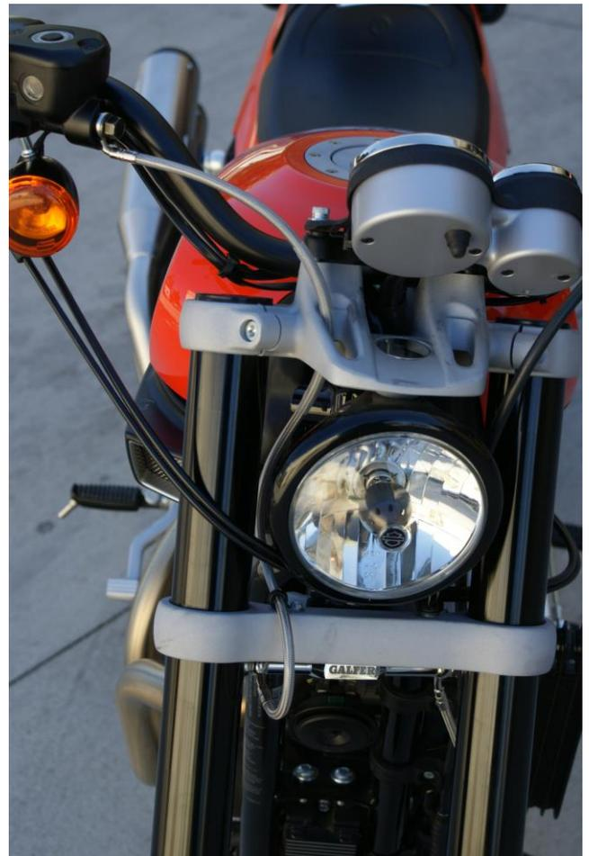
**c. Overall line A routing, behind throttle cables**
