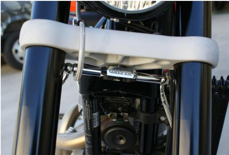
**d. Galfer union, under lower triple tree looking head on**
