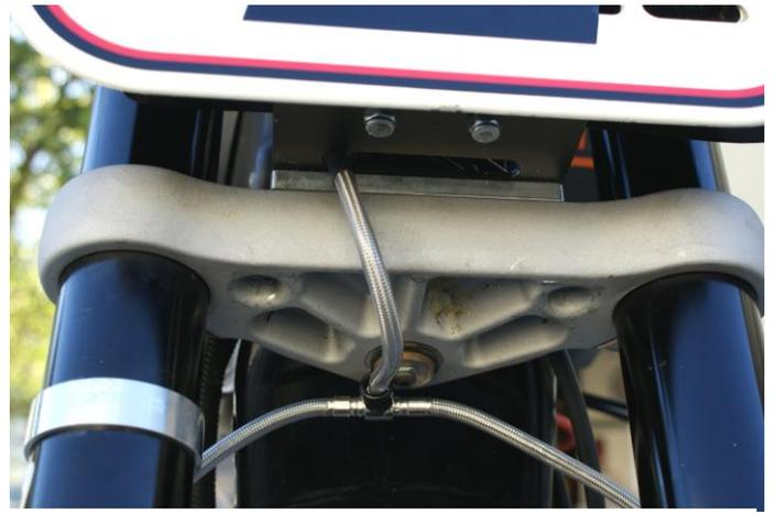
**B. Top line routing in front of lower triple tree, Galfer c-clip replacing union**
