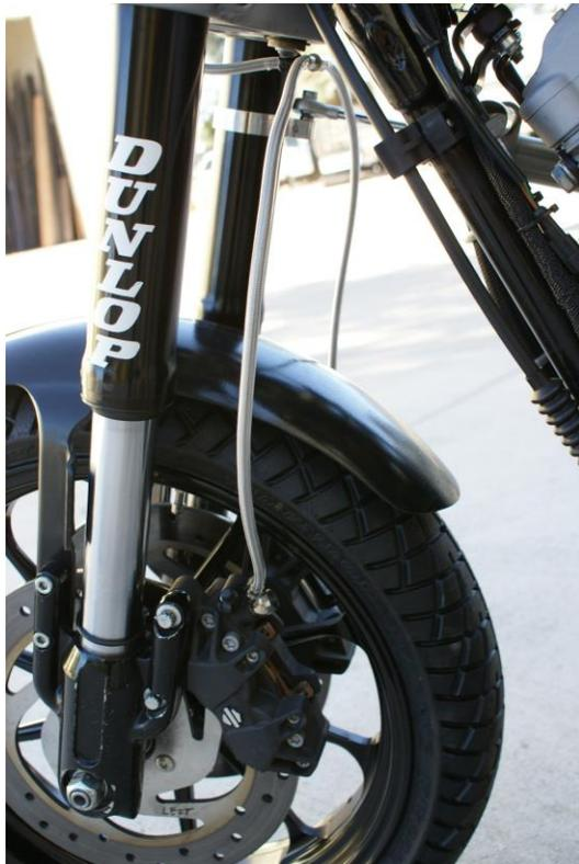
**C. Left and right line routing to calipers**
