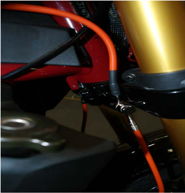
E. Lines D & E at Splitter Block
